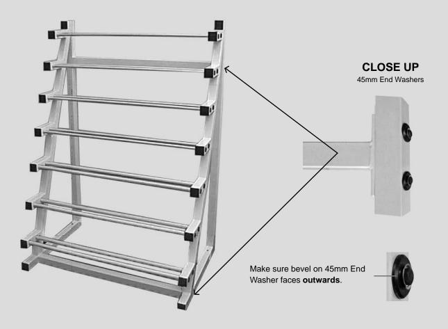
**Step 1:** When assembling, stand one leg up. Large holes should go to the **inside** of rack. It is easiest to assemble the rack by fitting bracing and tubular dumbell supports to one leg only complete and then repeat on the other side.
